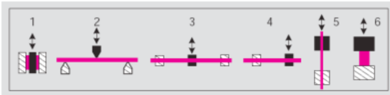
Fig. 1. DMA/SDTA861* measurement modes: 1 shear; 2 three-point bending; 3 dual cantilever (similar to bending but the sample is fixed); 4 single cantilever; 5 tension for thin bars, films and fibers; 6 compression. The clamping assembly is colored black and the sample red. The hatched areas show the parts of the clamping assemblies that remain fixed in position.
