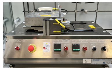
Film Applicator DeltaE (25-300 °C; speed 5-100 mm/s)
