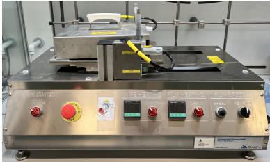
Film Applicator DeltaE (25-300 °C; speed 5-100 mm/s)
