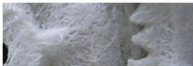
Fiber skeleton (as retrieved after burning off the resin)
