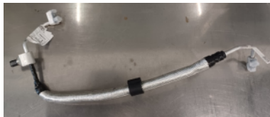
A/C refrigerant hose
